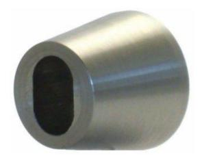
Milled from 40mm diameter mild steel bar Use with Morgan bullet lock SL001 Tapered profile to resist torque attack Self colour finish for excellent welding properties Fitted with zinc plated back washer Individually poly bagged
