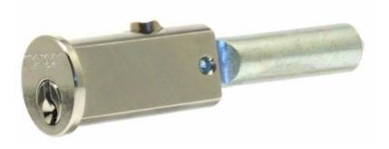
Extruded brass body, bright chrome plated Body size 22mm diameter x 14mm across flats, 46mm length Face dimensions 25mm diameter x 3mm Hardened steel zinc plated bullet 12.5mm diameter x 50mm length 5 pin tumbler mechanism 2 numbered keys Key blank TM15
