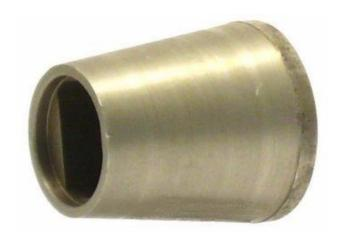
Milled from 40mm diameter mild steel bar
